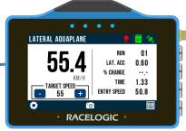
Results held on screen. Live speed continues. LEDs flash blue at bath exit. Target speed increments.
