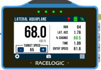
% change calculated: Max Lat. Acc. from test vs last run.
